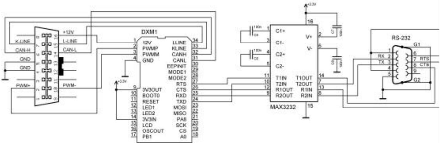
Schematic: DXM1 with FT232R USB converter
