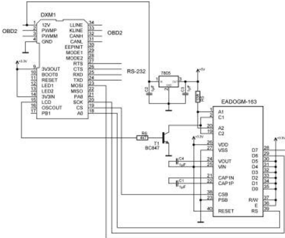
Connections of a LCD display (3 x 16 characters) to the SPI port of the DXM1.
