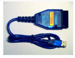
The DIAMEX DX35 interface is used for reading vehicle data that are provided via the OBD-II diagnostic port. The following items are included: the diagnostic interface and a software CD "moDiag-express". The interface translates the signals of the OBD-II diagnostic port into serial data which are understandable for the computer.
