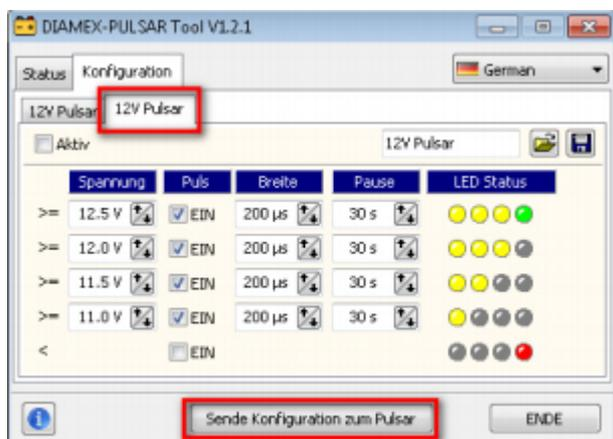
The pulse widths and intervals are adjusted in the following picture and the profile "12V Strong" was renamed. Through the button "Save Configuration" we secure the profile on the hard disk. By clicking on "active" the new profile will be activated and only needs to be sent to Tremex-PULSER. The new profile can be tested at the lead battery after removing the USB plug immediately.
